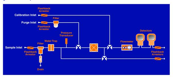
The system itself is self contained and simple to install. It is safe to use when sampling flammable gasses due to the inline flashback arrestors and internal cabinet gas monitoring.
