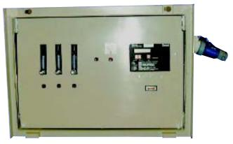
The system is designed to monitor hydrogen sulphide from three different locations at different concentrations simultaneously. For example, these could be the inlet, intermediate and output levels of a scrubbing system.
