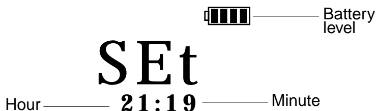
Figure 5: LCD in Time Adjustment Mode
