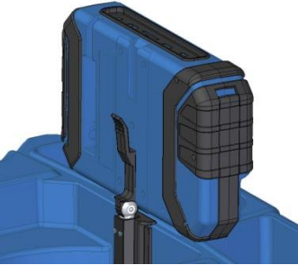
Fig. 71: Press lever and pull the monitor from the support at the same time.
