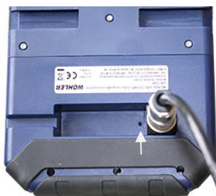
Fig. 69: Reset hole indicated by an arrow
