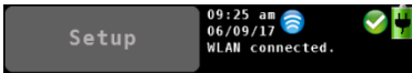
Fig. 35: „WLAN connected“ appears in the upper display, alternating with the selected customer
