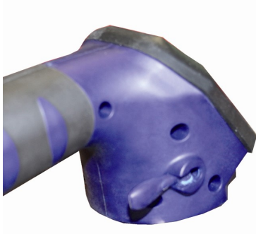
Fig. 18: Lever in vertical position - transport lock
