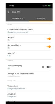
Changes to the measuring instrument settings in the app are transferred directly to the measuring instrument. Synchronization with the app is confirmed on the measuring instrument via "SYNC DONE".
