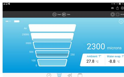
If the Vacuum probe is connected but that the measured values are beyond the measuring range, **"Atmo ↓"** is displayed:
