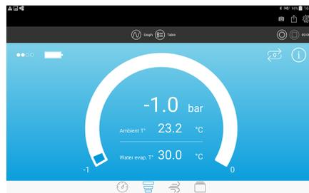
1. Perform an auto-zero, access to the connected probe information
