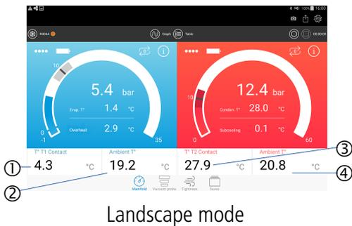
1. T° T1 contact: contact temperature probe 1
