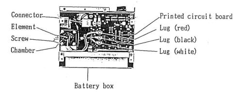
3) Draw out the connector from the printed circuit board. Take off three screws holding the battery box and take off the battery box. Set new battery box, front and rear panel plates as previous. When continuous operation time is less than greatly 4 hours for model GP-226 (In case of model GP-226,3 hours) after recharging of 15 hours, battery replacement is recommendable.
