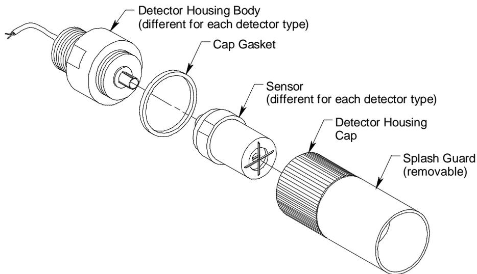
**Figure 2: 65-2300RK Toxic Detector Component Location**
