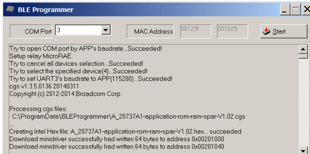
**Note:** Make sure the COM Port number is correct. If it is not, the procedure fails.
