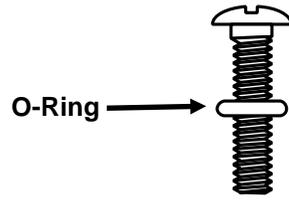
To prevent damage to the housing, the screw, and the O-ring, an electric screwdriver should be set with torque less than 3kgf.cm, and a speed rate of less than 670r/min.
