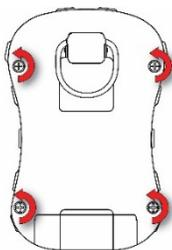
**Caution:** In some MicroRAE instruments a wire connects the buzzer in the top to the circuit board in the bottom. Do not damage or remove it.
