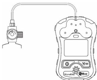
4. Connect the calibration adapter to the calibration gas.
