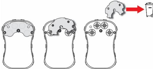
6. Set a new waterproof membrane filter on a flat surface. Peel off and discard one side's paper covering that protects the adhesive.
