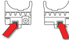
Align the Travel Charger with the middle of the MicroRAE, squeeze the latches on both sides of the Travel charger, and press it until it is firmly attached to the MicroRAE. Then release the latches. Make sure you press the latches close to the instrument instead of at their ends.
