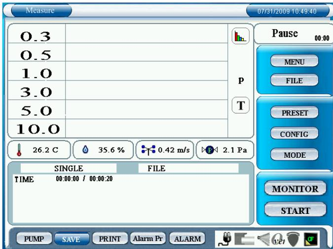
Tap [START] on the main screen to start a measurement in the setting configured in **3.5 MODE** and **3.7 CONFIG**.
