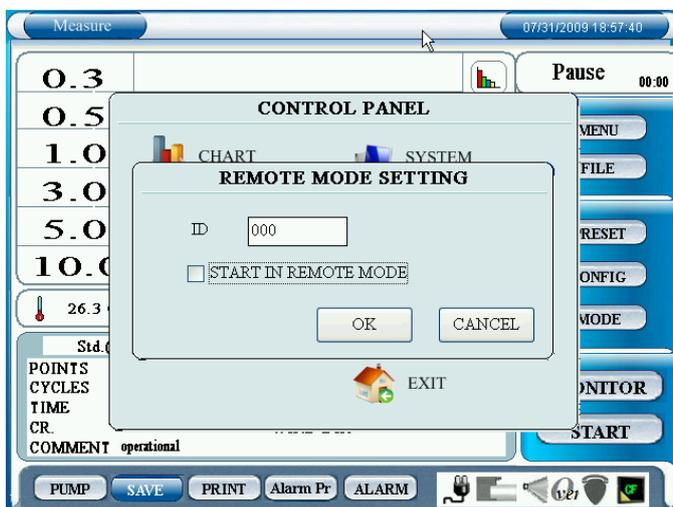
In the REMOTE MODE SETTING, check “START IN REMOTE MODE” to activate remote mode automatically when the instrument is turned ON.
