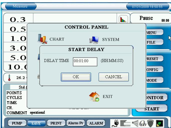
In START DELAY window set a measurement delay time.
