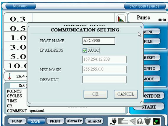
In the COMMUNICATION SETTING, configure the setting for Ethernet connection. This setting shall be configured when connecting the instrument to PC using remote console or remote mode.
