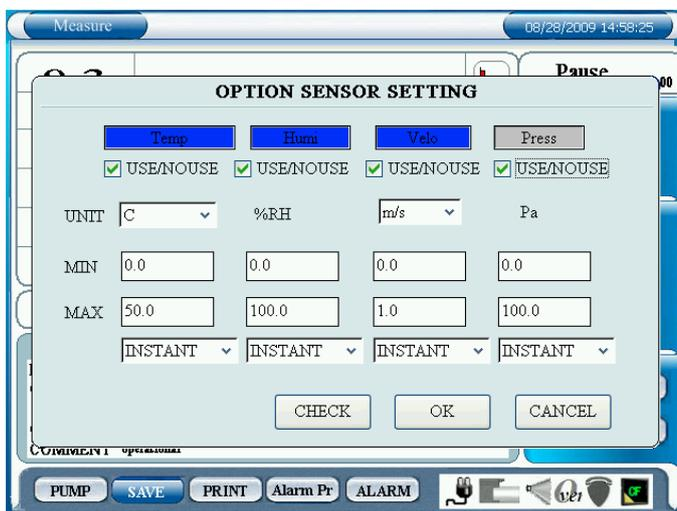
In the OPTION SENSOR SETTING window you can confirm if the option sensor is connected or not, and set to use or not to use the sensor. You can also set the unit and MIN/MAX range value for each sensor. MIN/MAX value should be the spec range for each sensor.
