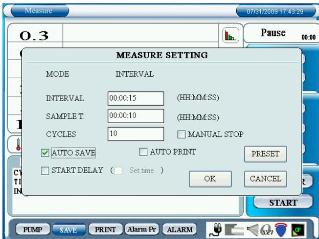
You can set INTERVAL, SAMPLE T., CYCLES and MANUAL STOP.
