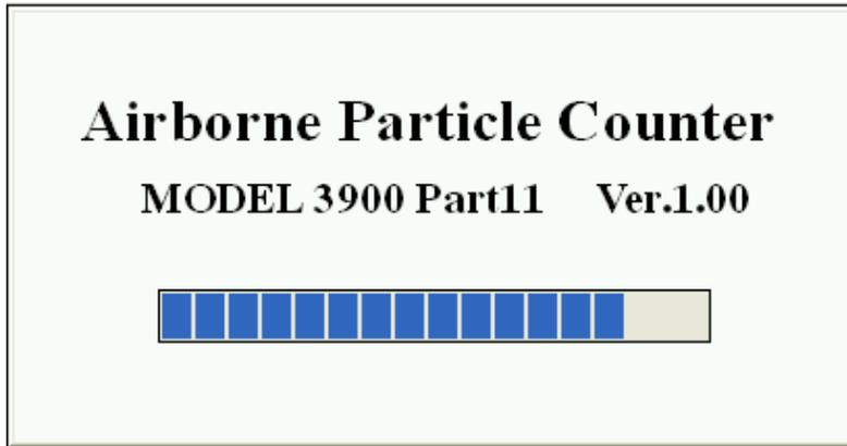
A few seconds after the instrument is turned ON, the screen shown on the left will be displayed.
