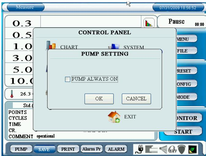
In the PUMP setting, set to turn the pump ON all the time or not.
