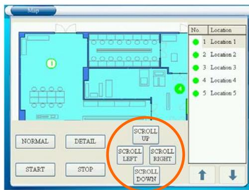
When a MAP is enlarged, [SCROLL UP], [SCROLL DOWN], [SCROLL LEFT] and [SCROLL RIGHT] buttons are activated, which enables you to move the MAP.
