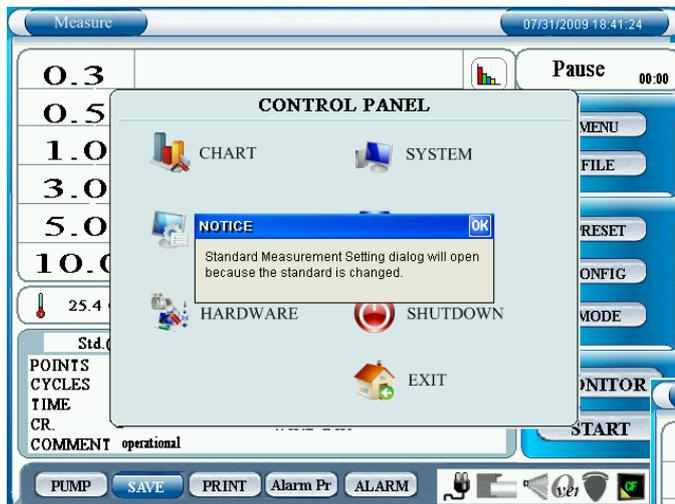
Change the settings and tap [OK] (Authentication required). Then a dialog will be displayed saying “Standard Measurement Setting dialog will open because standard is changed”. Tap [OK] at the upper right.
