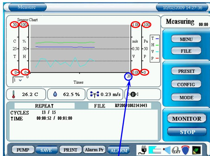
**MAX and MIN values** set for each sensor in the OPTION tab in the CHART SETTING window is applied in the chart. Tap **MAX or MIN value** to change it. (It changes in the order of MIN & MAX setting 1, 2, 3.)
