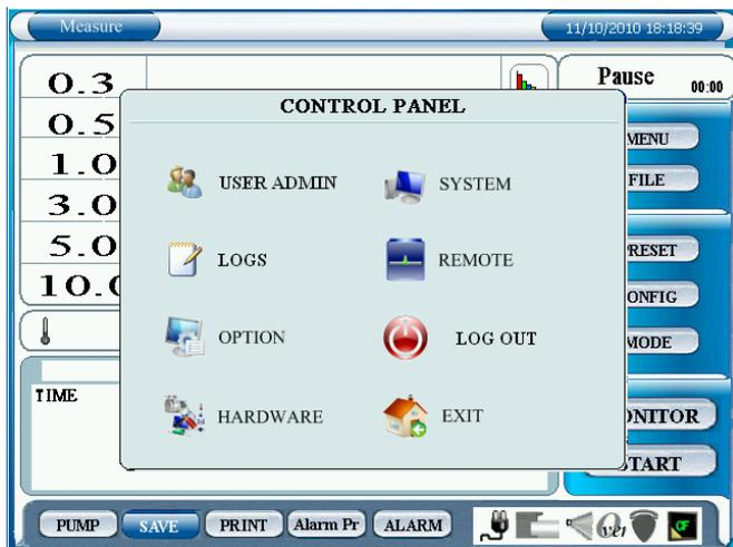
Select “MENU” on the initial screen to display the CONTROL PANEL window.
