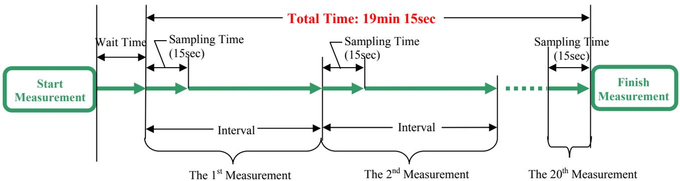
If the time period between two samplings is 10 seconds or longer, the pump will be turned OFF after a sampling is finished. Then the pump will be turned ON again 10 seconds before the next sampling starts.
