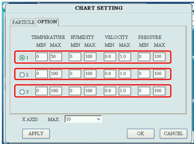
In OPTION tab, configure “MIN” and “MAX” settings for each sensor.
