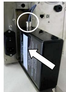
After supplying power using the power cord, switch ON the main power located on the rear of the instrument. When using battery, turn this switch OFF.
