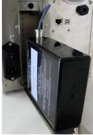
Open the battery compartment cover on the rear of the instrument. To open the cover turn the knob around 90 degrees. (Use a coin or something similar to turn it easily.)
