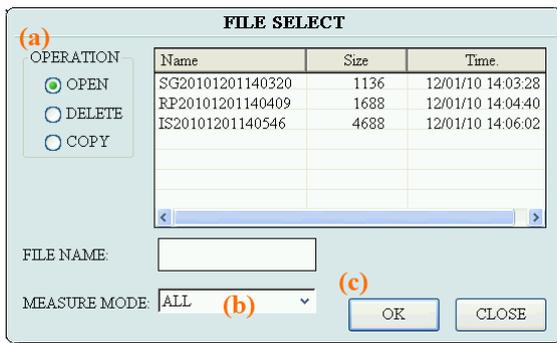
Select [FILE] on the initial screen. Then a screen shown on the left will be displayed. You can display, print and delete data here. You can also display the list of files that has been output in the ALARM/ERROR LOG screen.
