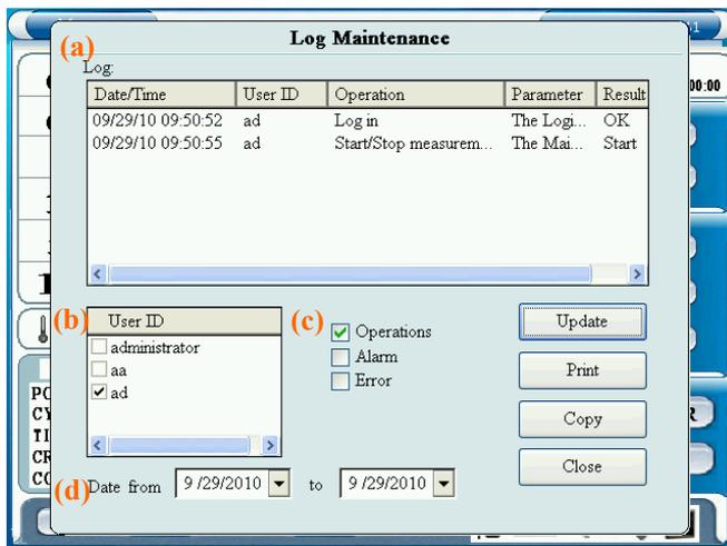
Log Maintenance window shows up when you choose “LOGS” on the control panel.
