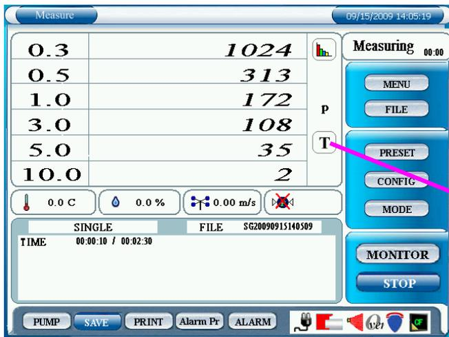
Tap **T** on the display with data for 6 particle size to switch to Single display.
