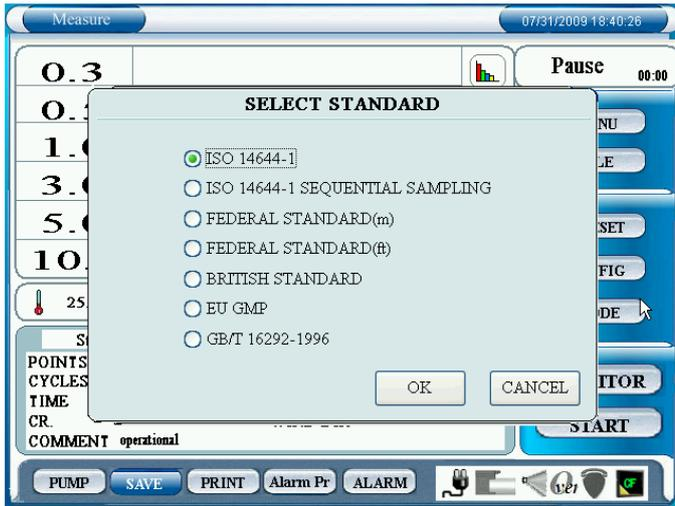
In the SELECT STANDARD window, select a measurement standard to be applied in the STANDARD mode.
