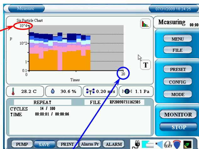
**MAX** value set in the PARTICLE tab in the CHART SETTING window is applied in the chart.
