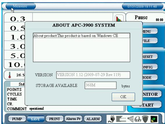
Tap [ABOUT] to view the firmware version of the instrument and remaining capacity of the internal data storage.
