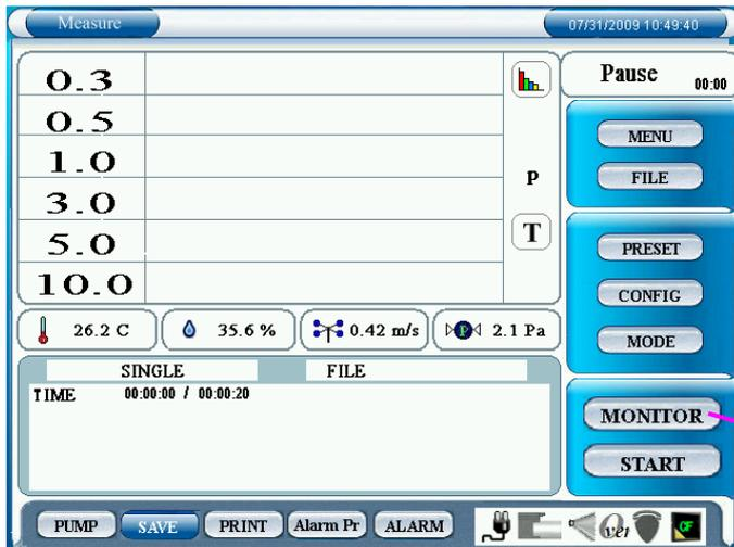
Tap [MONITOR] on the initial screen to start monitoring. Sampling will start in 10 seconds after the pump starts operating.
