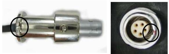
Insert the battery as shown on the right picture (the connector end should go to the rear of the compartment), and turn the knob back to the original location to close the cover.
