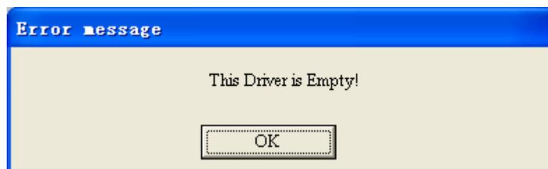
3) If there is a communication failure between the computer and the instrument, the following message will be displayed:
