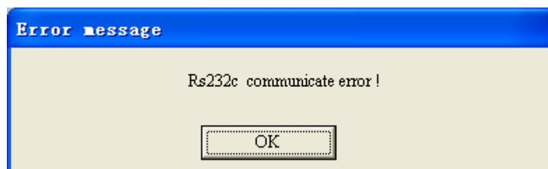
Confirm the communications cable is properly attached and the baud rate settings are correct.
