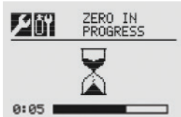
Figure 5. Zero Gas Calibration in Progress
