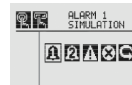
Figure 16. Alarm/Fault Simulation Menu
