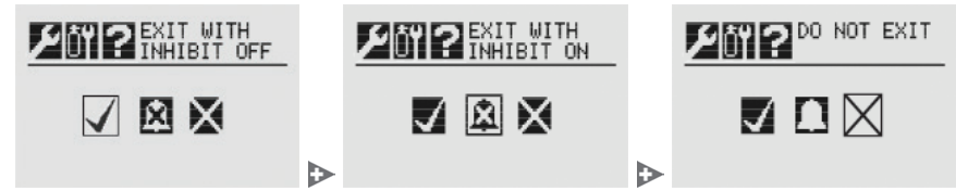
Figure 11. Exiting Zero Gas and Span Gas calibrations
