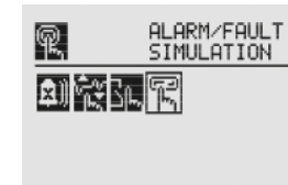
Figure 15. Alarm/Fault Simulation Screen
