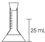
Add the content of one packet of **HI 93746** TPTZ reagent, close the cylinder and agitate for 30 seconds. This is the blank.
