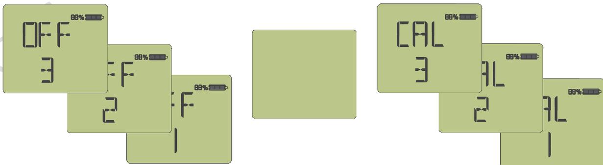
The detector will first automatically zero the sensors at the current baseline reading. Then the detector will prompt to "APPLY GAS":
