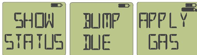
The detector will flash between "BUMP DUE" and "APPLY GAS". Apply gas to the unit at a flow rate of 0.25 to 0.5LPM using the calibration cap provided. Once all sensors have gone into alarm, the unit will return to normal operation (in alarm) and the bump due date will be reset.
