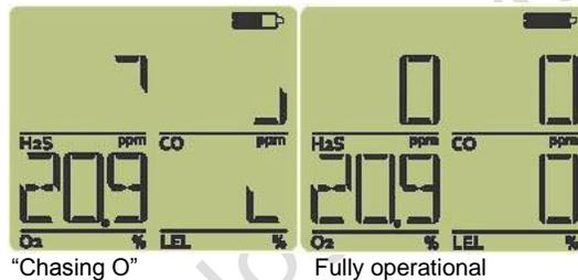
Once all sensors have completed the warm up sequence the detector is ready to detect all gases.
