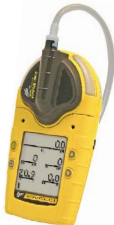
GasAlertMicro 5 with integrally attached pump
