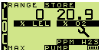
Fig. 4-10 H2S Sensor Fault
