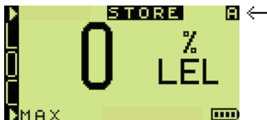
Fig. 3-33 Alarm Enabled Identifier
