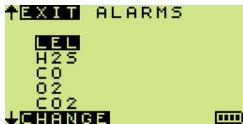
Fig. 3-7 List of Installed Sensor Types
