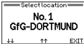
By pressing the left and centre button a stored place will be selected. The choice is automatically completed, when the selected value is confirmed with the right "Back" button.
