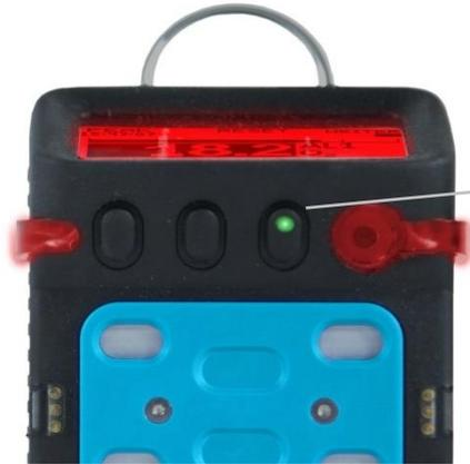
Switch on the device by briefly pressing the right button
