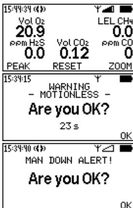
If the device user cannot act for himself any more, he can rapidly call for help by the acoustical alarm signalling or by radio.
