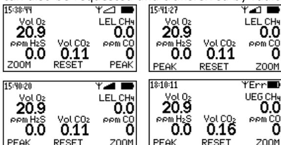
If the radio module is activated, the icons for radio and field strength are displayed in the upper display row. The stronger the field strength icon is filled in, the better is the radio connection. A flashing field strength icon signals that currently no measured values are requested or that the radio connection is interrupted. If the icon is displayed, the radio module is either defective or switched on but not existing at all.
