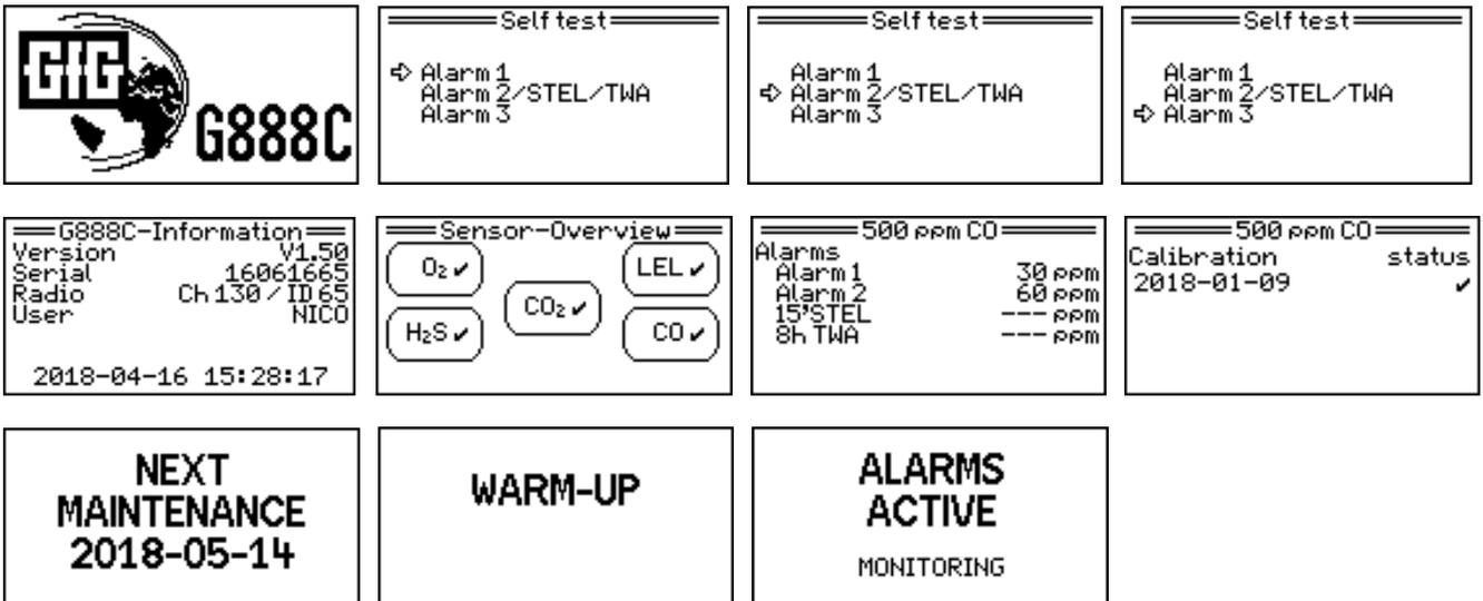
Alarm thresholds and calibration data will be displayed for all available sensors. Please find an example of CO below. Depending on the condition of the sensors, other messages will be output, which possibly need to be acknowledged. Please find more detailed information in the section "Other messages when starting the device".
