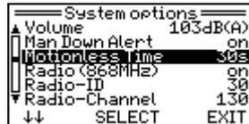
The "Motionless time" can be set from 20...300s. After the expiration of this time, the device user will be warned for 30 seconds. Only afterwards, the "Man-Down-Alarm" will be triggered in the measuring mode.
