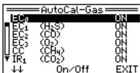
Here it is possible to set which sensors should be calibrated for the automatic adjustment with test gas. By default, all sensors are set to "OFF". If several sensors need to be adjusted simultaneously with a test gas mixture, these sensors can be selected here.
