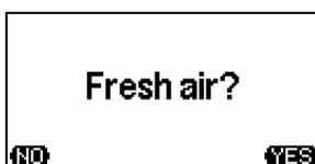
Only if it is made sure that **there is no flammable gas on the sensor, but only fresh air, the question may be answered with YES**. In this case, the sensor will be reactivated and will display measured values after a short running-in period!
