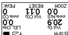
The G888 allows turning the measured value display by 180°. To do so, keep the left and right button pressed simultaneously and release it. In this way, the display can be easily read when the device is attached to the belt.
