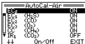
Here it is possible to set which sensors should be used for the automatic adjustment with fresh air.
