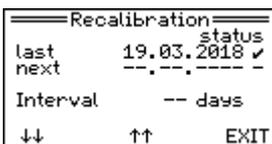
Sensor adjustment on March 19th, 2018 was correct. The interval of the functional test is not activated.
