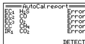
AutoCal adjustment with test gas mixture has not been successful. (e.g. due to wrong test gas concentration)
