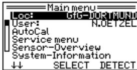
From a table stored in the device, it is possible to select one of 100 possible places. All table entries can only be edited with a PC. In a table entry it is possible to save up to 15 letters / figures, which are saved as "**Job site**" in the G888.
