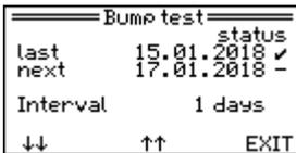
Interval of the functional test is activated; the next functional test is immediately due.
