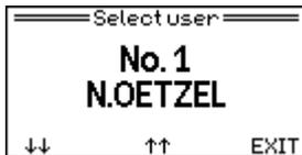
By pressing the left and centre button a stored user will be selected. The choice is automatically completed, when the selected value is confirmed with the right "Back" button.
