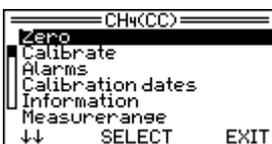
The individual data of the sensors which are built-in the device, are displayed here.
