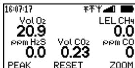
It is possible to continuously display peak values in the peak mode which is activated by pressing the button **PEAK**. On the screen in the top row, the peak icon  $\nabla$  will be displayed with the two arrows.
