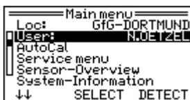
From a table stored in the device, it is possible to select one of 20 possible entries. All table entries can only be edited with a PC. In table entries it is possible to save up to 15 letters / figures, which are saved as "**Identification**" in the G888.
