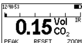
In order to be able to see the measured values magnified on the **Zoom** display, press the **right button (ZOOM)**. Briefly press the button in order to zoom a displayed value. By pressing the right button several times, you can zoom the display of the measured values of the individual sensors one after another.
