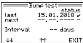
Interval of the functional test is not activated.
