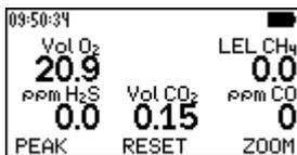
The G888 is ready for operation if the time, the battery icon and all measured values are displayed with the measuring gas and the unit. It is monitored if the measured gas concentrations exceed the preset limit values and in case of oxygen it is monitored if the measured values fall below the preset limit values.
