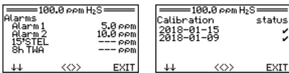
The data of the last three sensitivity adjustments can be displayed in the sensor menu "Calibration data". The status display indicates if they have been successful (✓) not faulty (✗).
