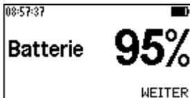
In the measuring mode, the capacity of the battery can be read from the state of charge battery icon on the right of the display. The black filling represents the remaining capacity. By pressing the right button (**ZOOM**) several times, if required, it is also possible to display the remaining capacity as a figure. (\*1)
