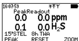
In the detail view of the zoom display on the top left the corresponding peak value is displayed instead of the max. or min gas concentration.
