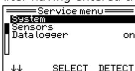
In the menu item **System** it is possible to perform general settings (refer to the section "System menu"). In the menu item **Sensors** it is possible to set sensor-specific functions (zero point and sensitivity adjustment). It is possible to retrieve information or to set alarm thresholds. By pressing the button **DETECT** you would exit the service menu and go back to the measuring mode.
