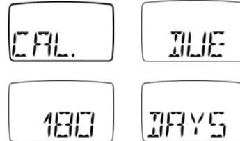
The LCD displays the number of days remaining before the detector must be calibrated. For more information, refer to [Calibration Procedures](#).
