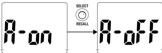
When the alarm is ON, press the SET button to save the setting and move to CO<sub>2</sub> alarm setting.
