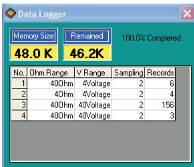
Click on one of the numbered files and the “Input Starting Time” box appears. Enter the exact time and date of the first reading in the file. The software will then put a time and date stamp on all of the records in the file. The data will automatically download at this time.
