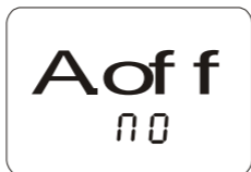
Figure 8: Disabling the auto off function
