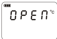
Figure 5: Display when no probe is detected
