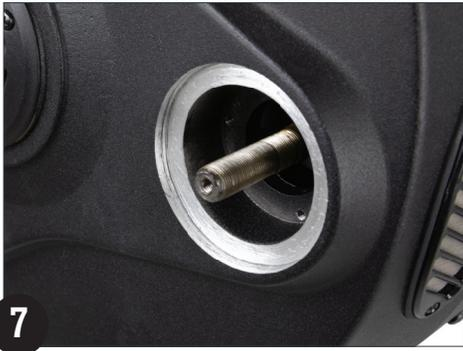
Unthread and remove the brass bushing from the focus shaft.
