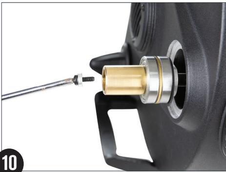
Thread the included retaining screw and retaining washer onto the end of the focus shaft until tight. The end of the focus shaft will be recessed within the focuser's brass cylinder.
