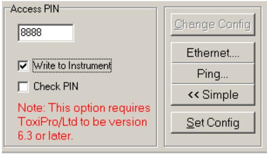
7. Enter a unique 4-digit PIN in the input box under Access PIN and click on "Write to Instrument".
