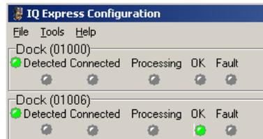
If a fault is detected and the IQ Express Dock is unable to complete the tests, the red fault light will be lit on the screen. Details of the fault will be listed in the input box on the right side of the screen under the instrument tab. See section 3.2.2 for details.
