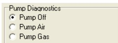
Click "Pump Gas" to draw span calibration gas through the right gas port at the back of the dock. Click "Pump Air" to draw the fresh air sample through the left gas input port.
