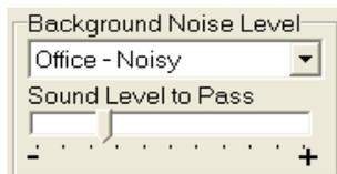
The Background Noise Level adjustment offers four levels of background noise levels. For the best results, select the one that most closely approximates the background noise level expected during testing.
