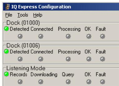
For docks in Listening Mode, if a single fault is detected on any of the docks, the dock LED will turn grey and the Fault LED will turn red.
