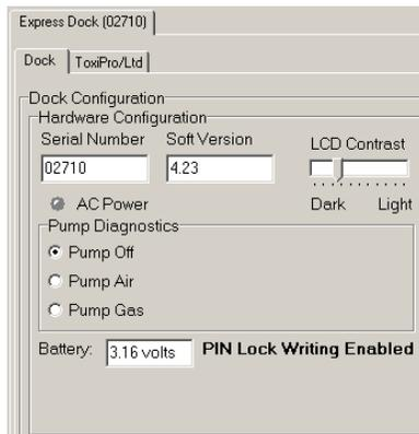
9. Place the instrument(s) that is/are to be configured with the PIN in the dock while PIN Lock Writing is enabled.
