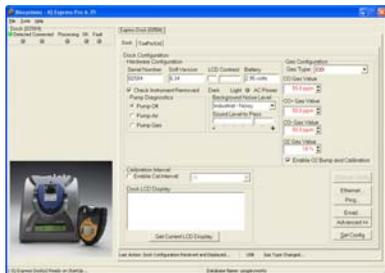
The screen is divided into right and left sides. The left side gives the status of the docks that are currently installed and recognized. At the top of the right side of the screen there is a tab for each dock that is currently installed and recognized. Within each dock tab are two sub-tabs: one for dock controls and one that shows the calibration status and details for the instrument that is currently in the dock.
