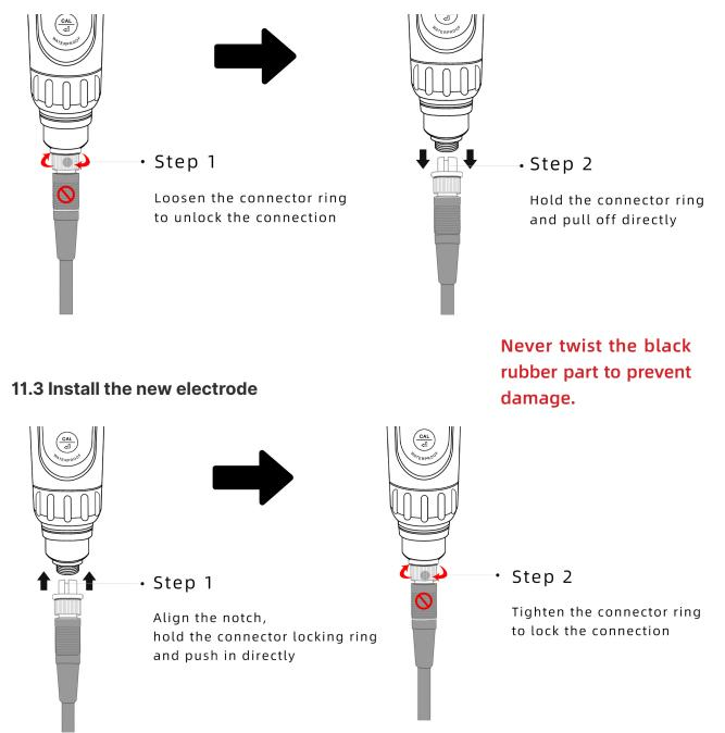
**11.4** After installing the new electrode, please at least perform a 2-point calibration. Refer to Section 4.1 for how to calibrate.
