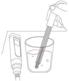
5.1.3 If necessary, turn on the Auto-Hold function (refer to Section 8.3.3), the reading will be automatically locked when it's stable for more than 10 seconds. Short press (CAL) to cancel the Auto-Hold and keep measuring.
