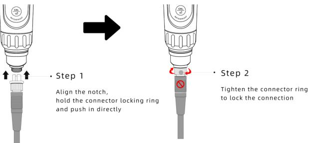
**11.4** After installing the new electrode, please at least perform a 2-point calibration. Refer to Section 4.1 for how to calibrate.
